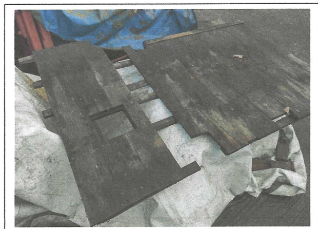
The last footplate flooring, reference used for placement of the joists
