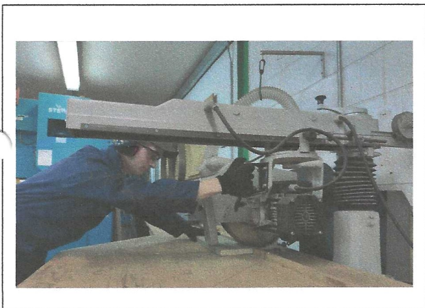
Myself using the Radial arm saw to cut the timber
