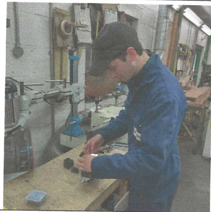
Myself setting up Spindle moulder cutting block
