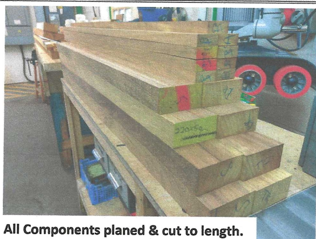
Timber cut into smaller lengths ready to be cut length ways.
