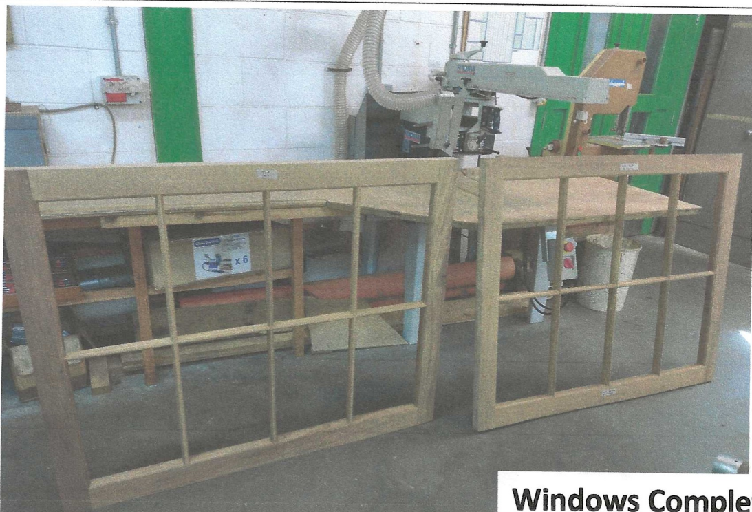
Window cleaned with 180 grit sandpaper. Prepared for painting.
