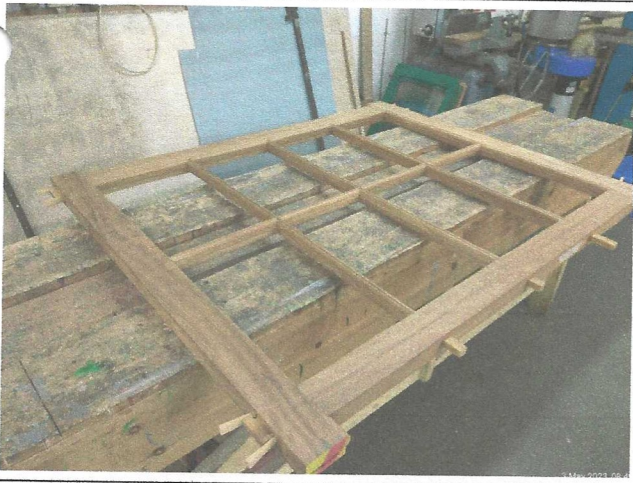
First window wedged and glued ready for the horns to be cut.
