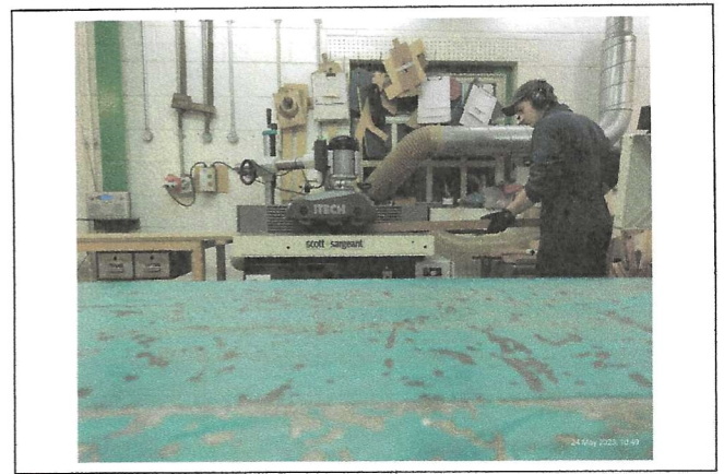
Cutting rebates on spindle moulder
