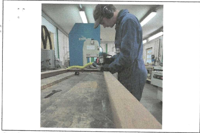
Cutting Half Round on inside edge of the frame
