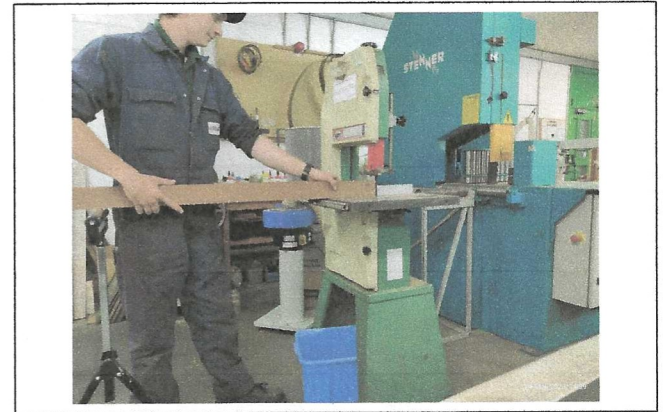
Cutting Tenons on bandsaw
