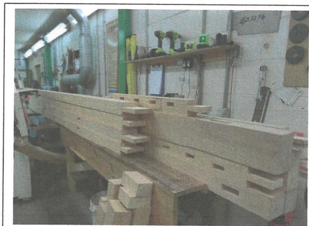
All Tenons & mortices cut ready for dry assemble
