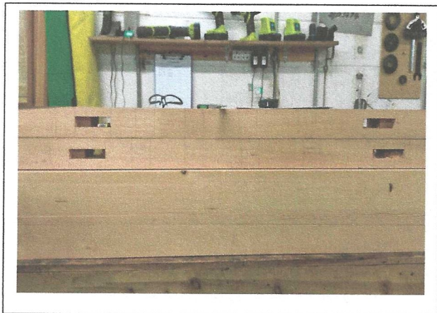
Four cut Haunch Mortices & 8 marked out mortices
