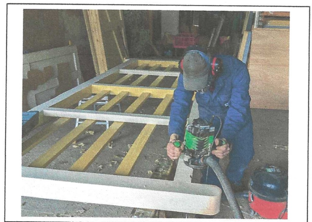
Myself using a router to cut the chamfered edge
