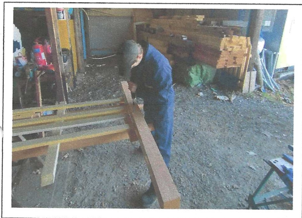
Myself drilling holes for dowels
