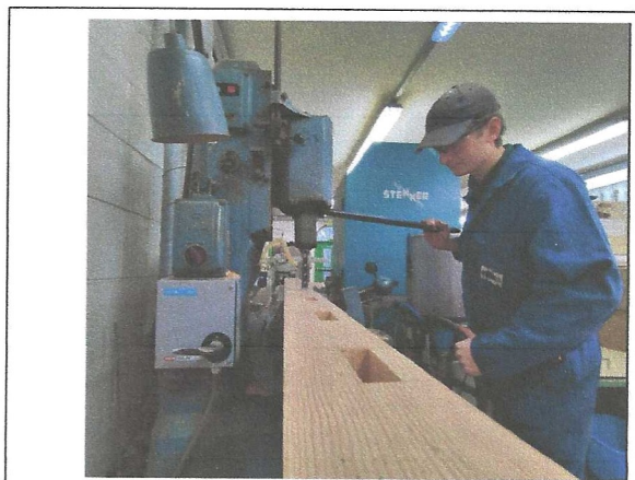
Myself cutting mortices using Morticer.
