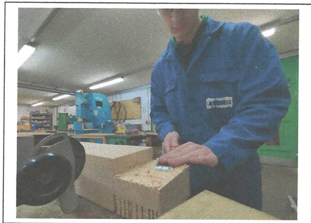
Myself cleaning up tenon after cutting tenon with Radial arm saw
